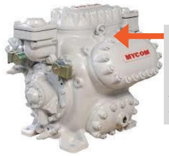
Reciprocating compressors can often be used in refrigeration applications and rack systems with multiple compressors. It is important to record the model numbers of any additional oil reservoirs and to identify any refrigeration lines that run for more than 75' from the compressor to the condenser.
